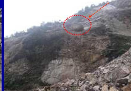
**Rock-fall Type 2: Sliding and subsequent rolling of rock blocks**
