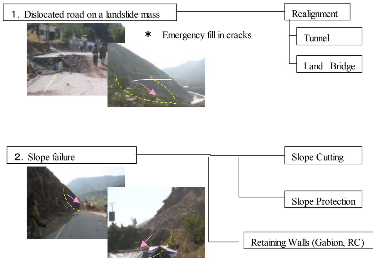
**Figs. 12 and 13.** Basic measures for slope failures
