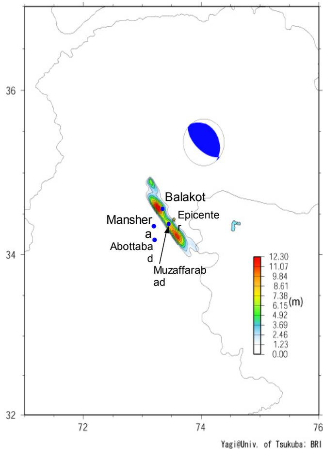
Fig.1. Source Process of Pakistan earthquake: contours show the slip on the fault surface ([http://www.geo.tsukuba.ac.jp/press\\_HP/yagi/EQ/2005Pakistan/](http://www.geo.tsukuba.ac.jp/press_HP/yagi/EQ/2005Pakistan/))
