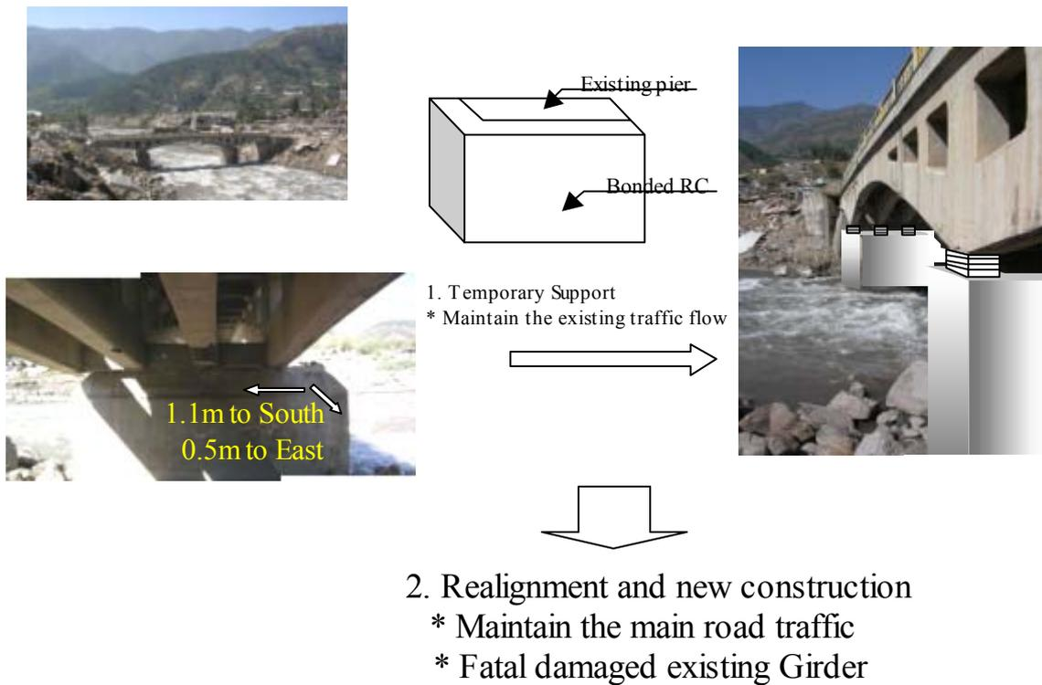
**Fig. 15.** Rehabilitation of Balakot bridge
