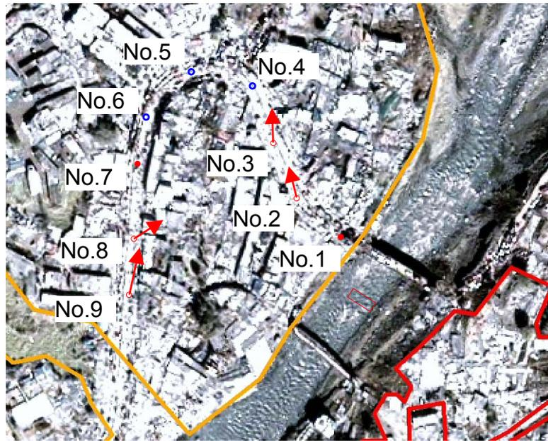
**Fig. 7.** Location and the inclination of the lampposts (●: sound, ○: shaky, ○: bent). Arrows show the direction and the amount of the inclination (20degree=1cm). Imagery taken from UNOSAT website (<http://unosat.web.cern.ch/unosat/asp/>)
