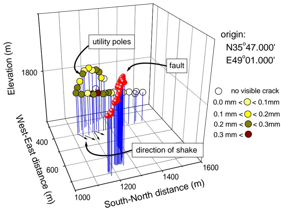
**Fig. 1.8** Locations of cracked utility poles
