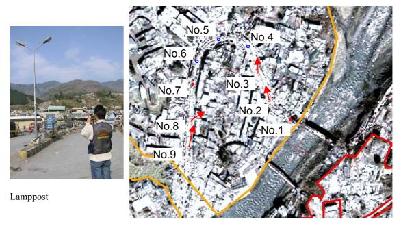
**Fig. 7**. Location and the inclination of the lampposts (●: sound, O: shaky, O: bent). Arrows show the direction and the amount of the inclination (20degree=1cm). Imagery taken from UNOSAT website (<u>http://unosat.web.cern.ch/unosat/asp/</u>)
