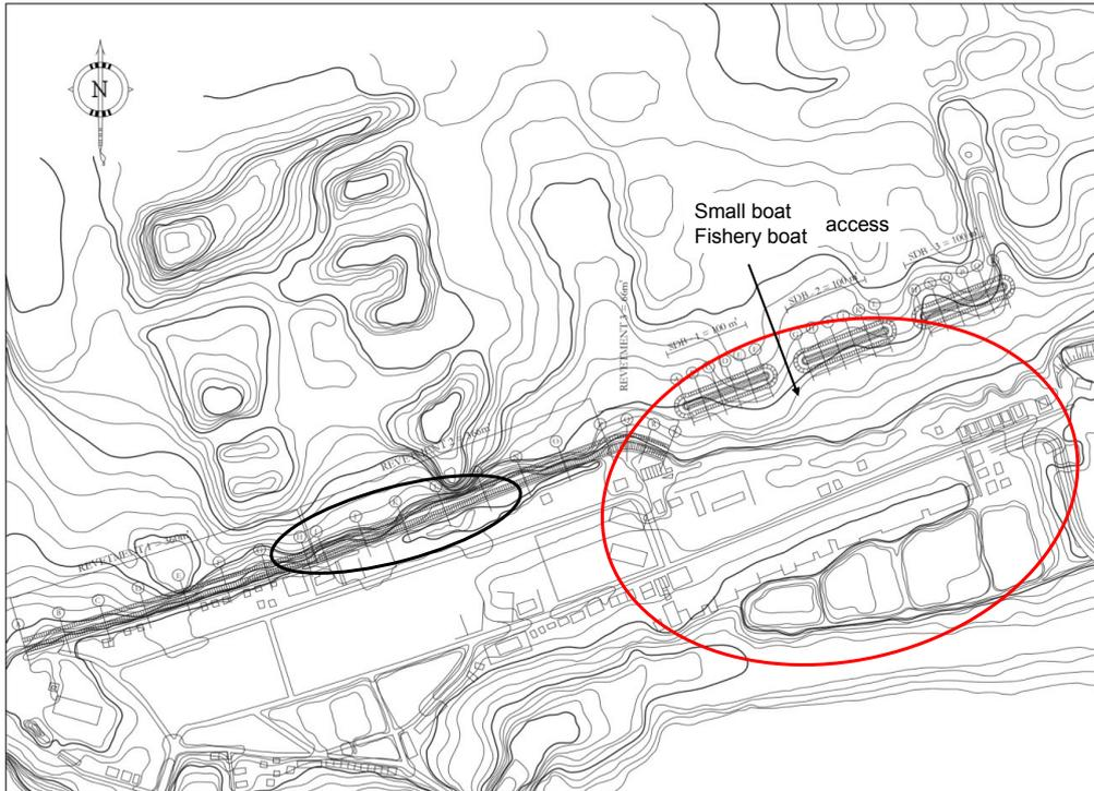
Figure 10.4 Plan view of the revetment and the submerged breakwater
