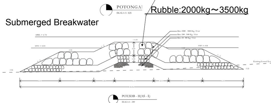
Figure 10.5 Cross section of revetment and submerged breakwater
