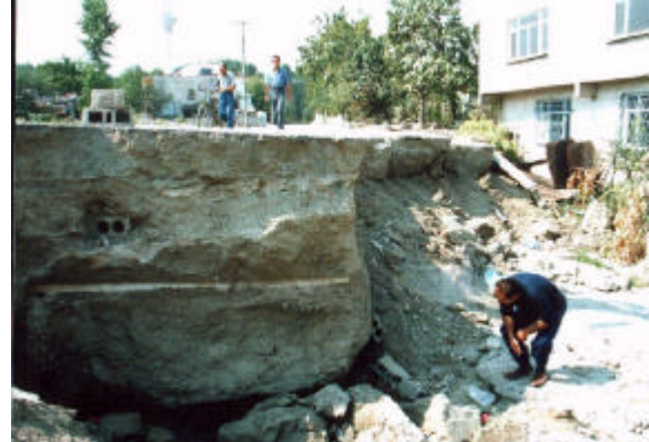
Figure 4.13 Normal faulting in Kavaklı (Gölcük)
