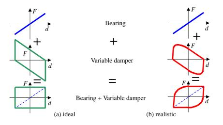
Figure 2. Ideal and realistic hysteretic loops produced by pseudo negative stiffness damper
