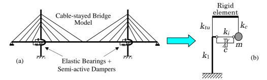
Figure 1. Simplified model for the cable-stayed bridge
