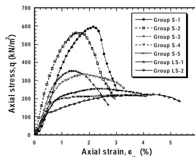
Figure 3. Typical stress-strain relationships of each group.
