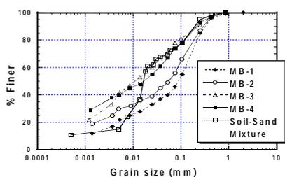
Figure 1. Grain size distributions of old adobe and soil-sand mixture used in this study.
