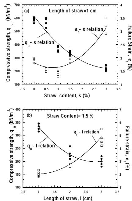
Figure 4. Relationships of (a)  $q_u \sim s$  and  $\epsilon_f \sim s$ , (b)  $q_u \sim l$  and  $\epsilon_f \sim l$ .
