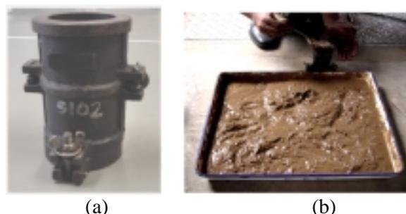
Figure 2. Photograph of (a) a typical mould used for sample preparation and (b) pouring of mix in a mould.
