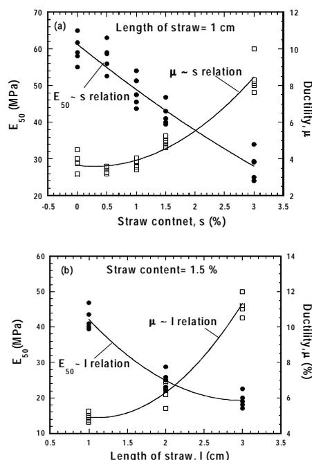
Figure 5. Relationships of (a)  $E_{50} \sim s$  and  $\mu \sim s$ , (b)  $E_{50} \sim l$  and  $\mu \sim l$ .
