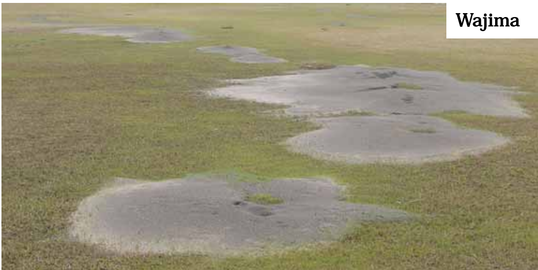
Figure 8.3 Some examples of liquefaction and its effects
