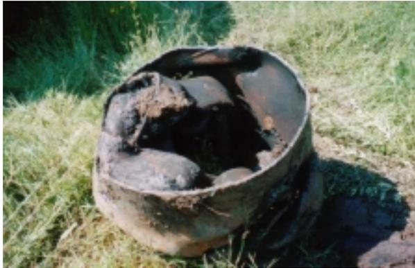
Figure 8.2 Buckling of water supply steel pipe
