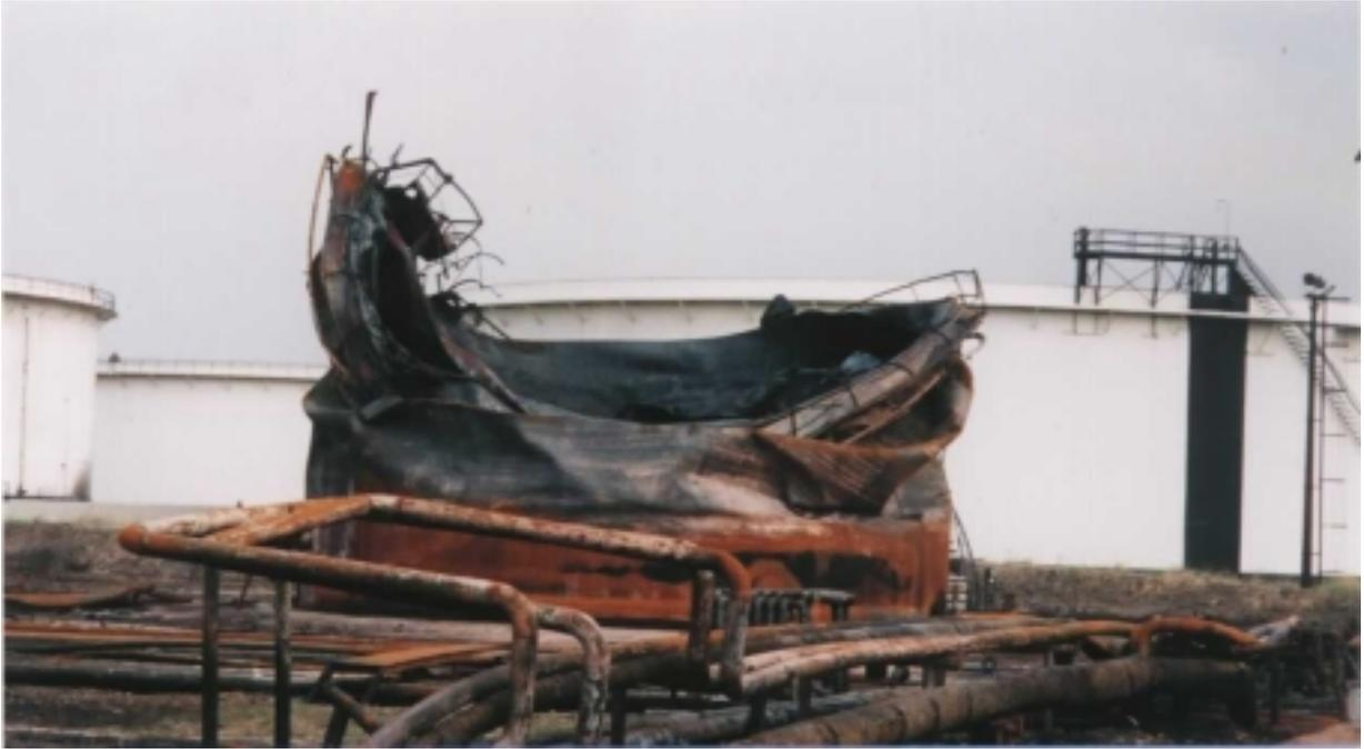
Figure 7.3 Burned cylindrical tank
