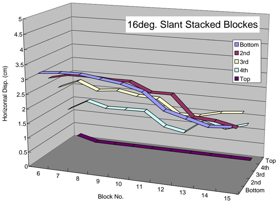
(b) Horizontal displacement of blocks (16 deg. Slant stacked model)
