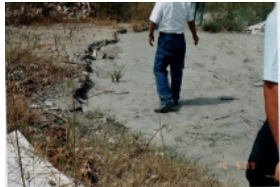
Photo.8.17 Boiled sand around fissure
