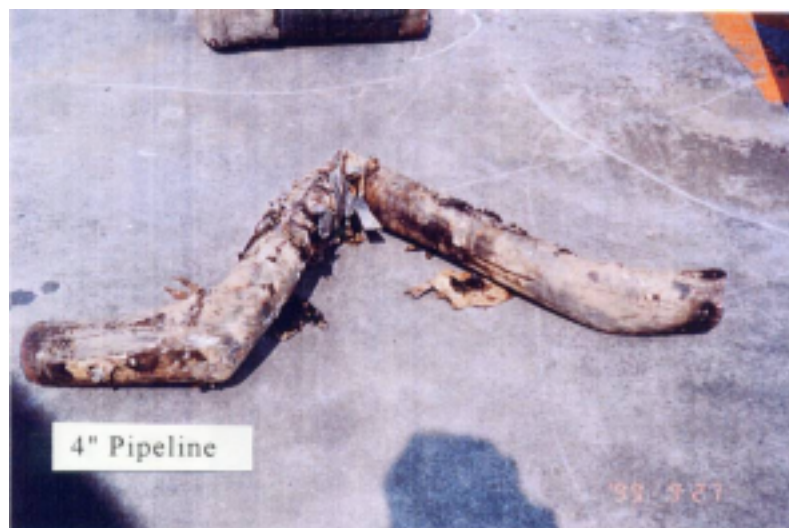
Figure. 7.25 The rising of the road surface and the deformed 8" and 4" pipes
