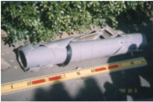
Figure.7.41 Push in each distribution pipe (vinyl pipe) at joints (Displacement is about 0.8m)
