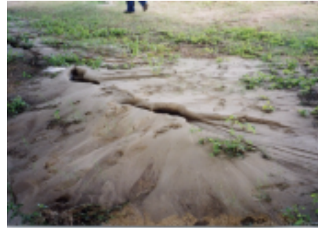
Photo 4.33 Trace of liquefaction
