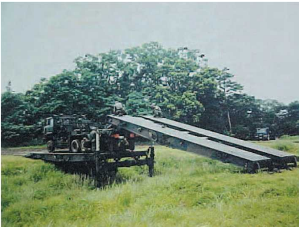
Photo 2. Type 81 self-propelled bridge (bridge length: 10 meters per span, height: up to 4 meters, width: 3.75 meters, capacity: 50 tons)
