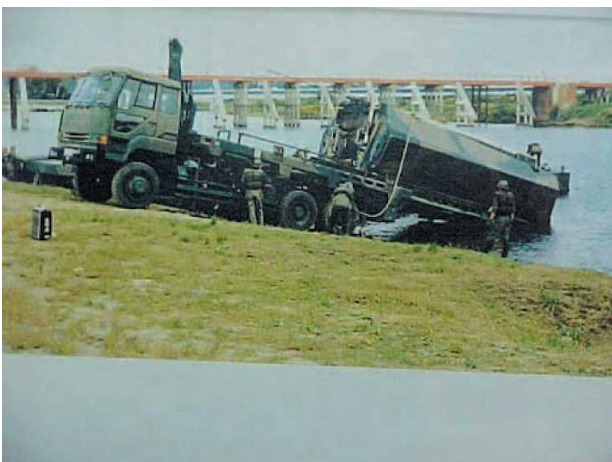
Photo 3. Type 92 heavy pontoon bridge (bridge length: 10 meters per span, width: 4 meters, capacity: 50 tons)
