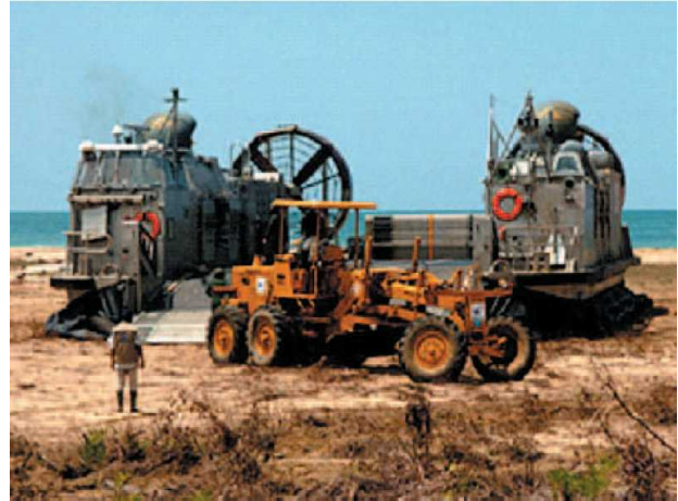
Photo 1. Air cushioned landing craft (standard displacement: 85 tons, speed: 40 knots)
