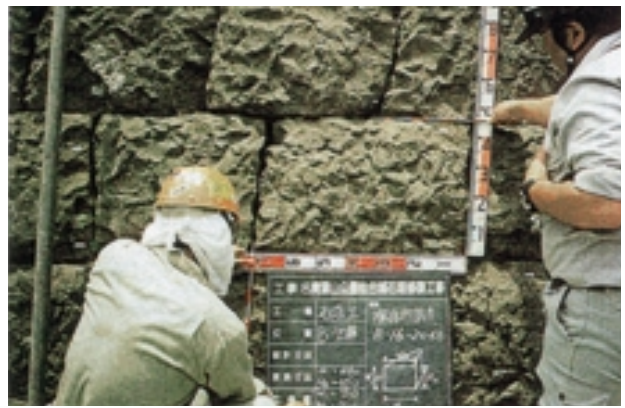
Photo 2 Measuring dimensions of stones
