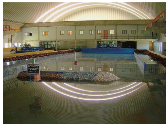
Photo 9: Experimental wave tank of the MTI (June 2004) (The wave generators in the front were provided from Japan)
