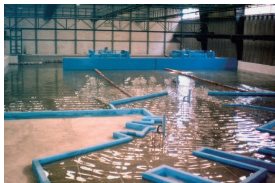
Photo 5: Hydraulic model experiment at Mexico Port Hydraulic Center (November 1987)
