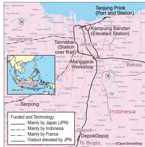
Figure 1: Improved Railway Lines currently in use in Jabotabek Project (Double Tracking, Electrification, and Automatic Signaling)
