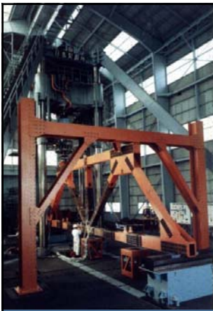
1/4 scale model of truss
