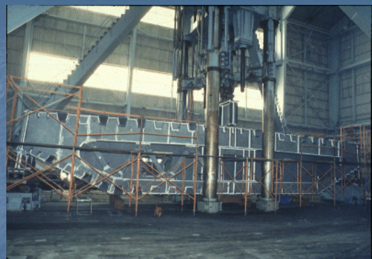
Full scale Box girder section fatigue test
