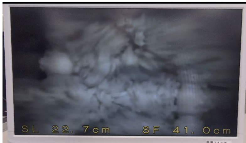
Fig. 3 AI slump-prediction system in operation
