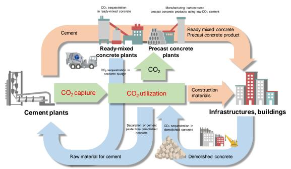
Fig. 4 Carbon recycling technology for the cement industry (supported by New Energy and Industrial Technology Development Organization)
