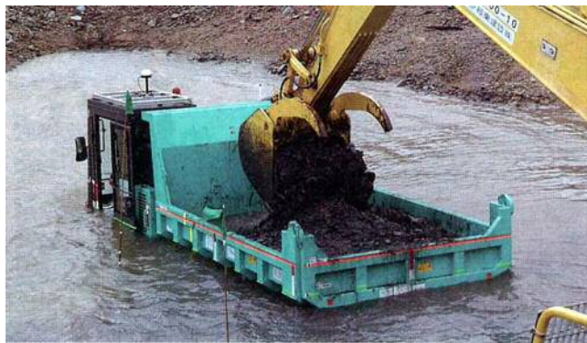
Photograph 2. Remote-controlled semi-submersible heavy load tracked-transporter.
