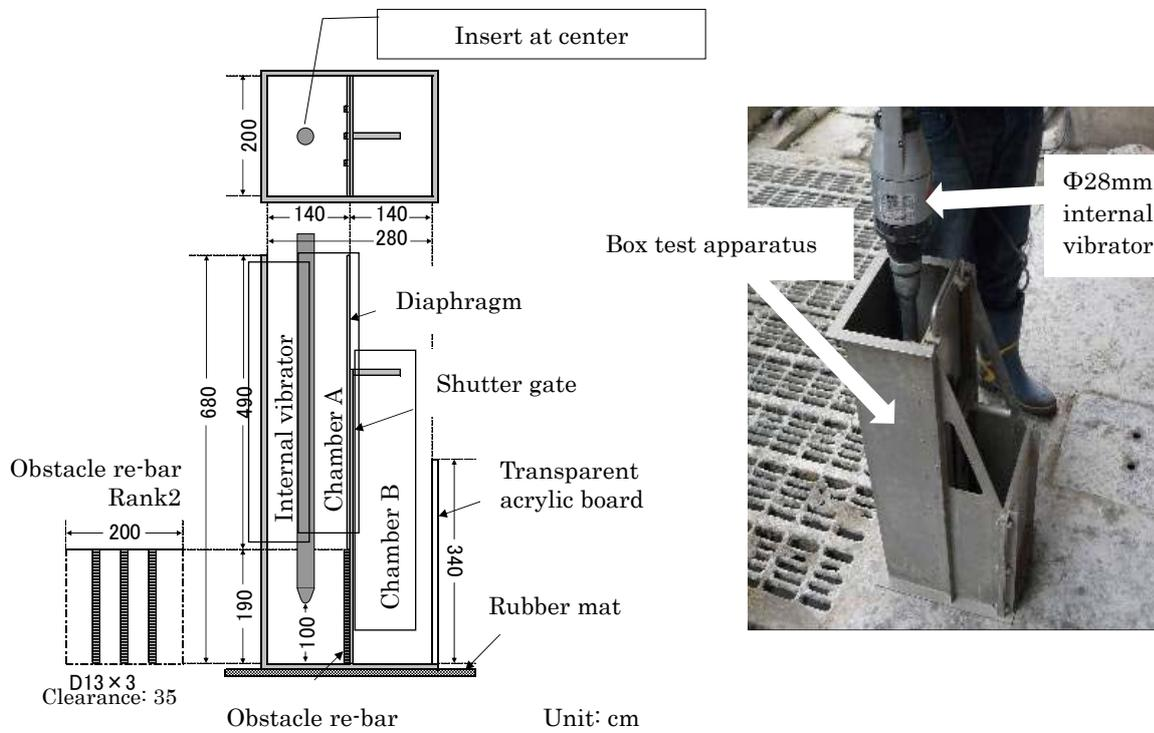
Fig. 4 Schematics of draft passability test method with vibration
