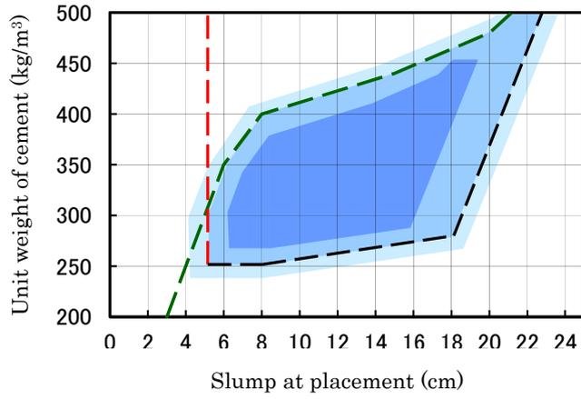
Fig. 3 Relationship between unit weight of cement and suitable slump
