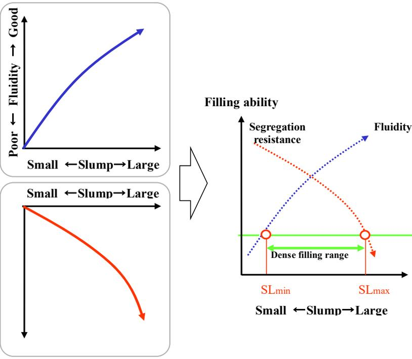
Fig. 2 Influence of the slump on filling ability
