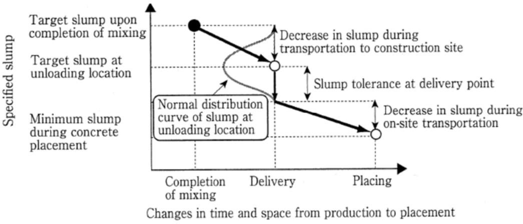
Fig. 1 Relationship between specified slump at each stage of construction and decrease in slump
