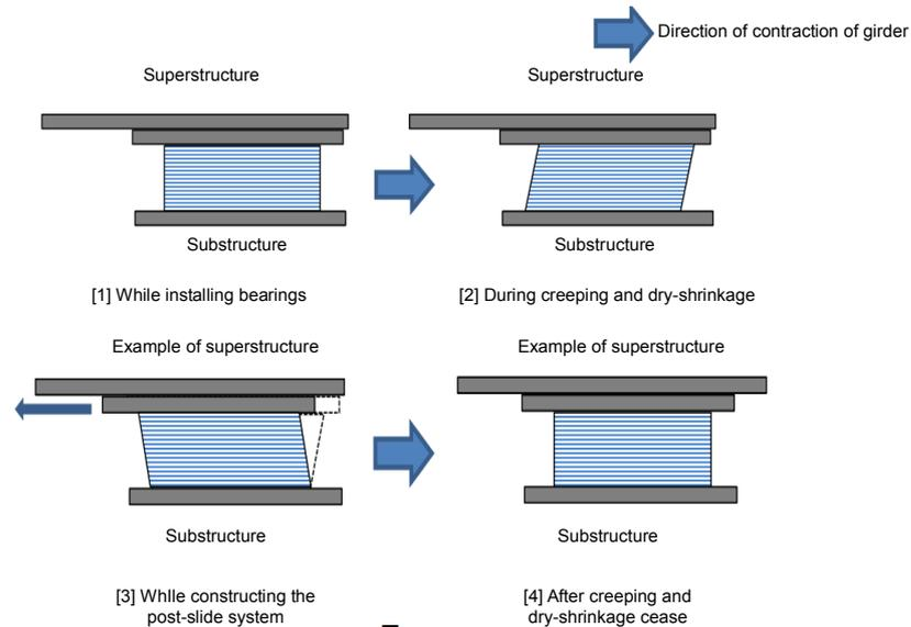
Figure 4. Construction procedures for post-slide system
