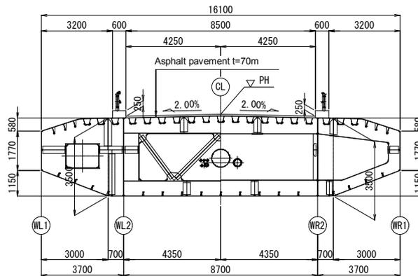
Figure 3. Section of the main line section
