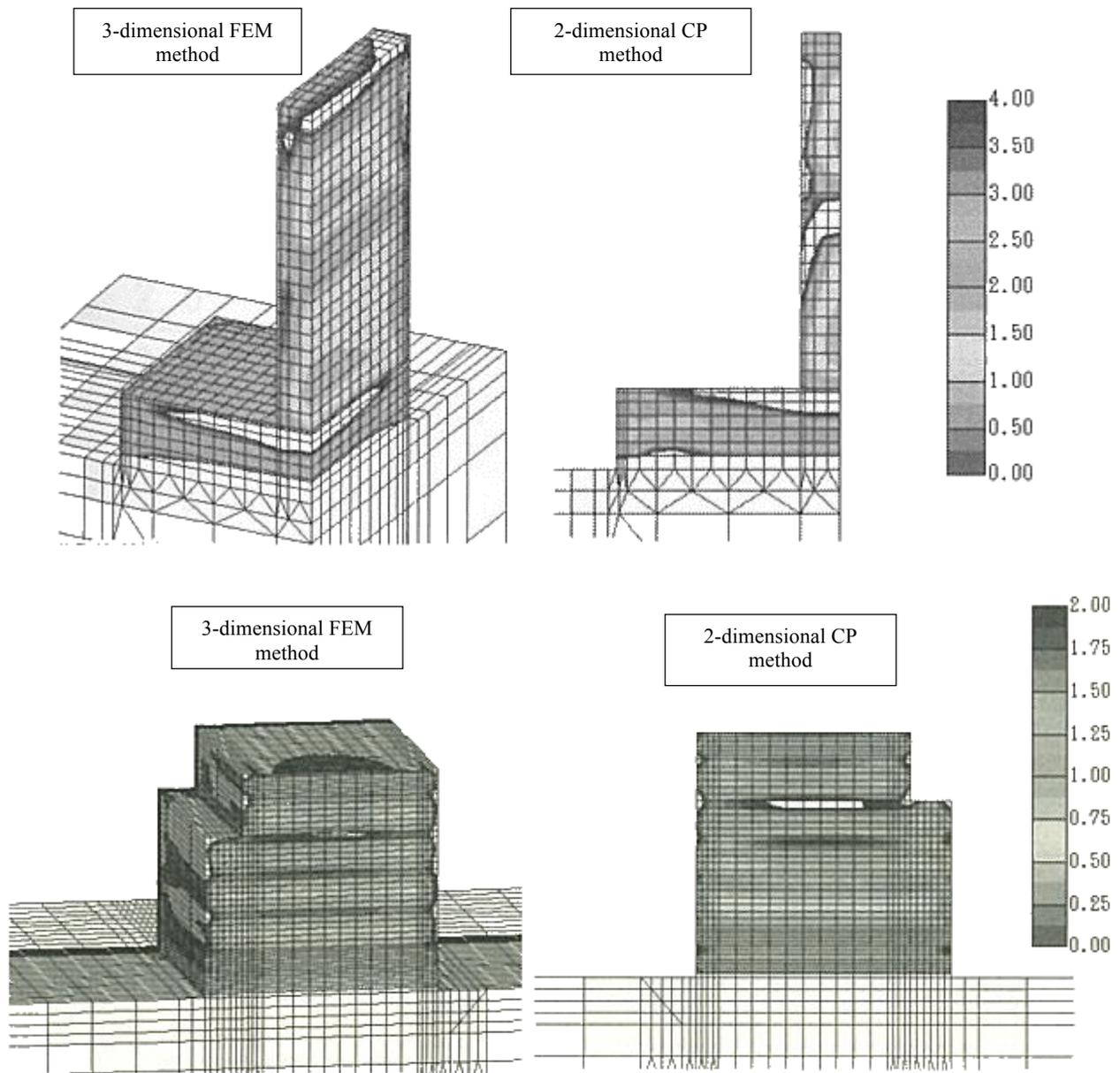
Fig. 2 Contour diagram of minimum crack width
