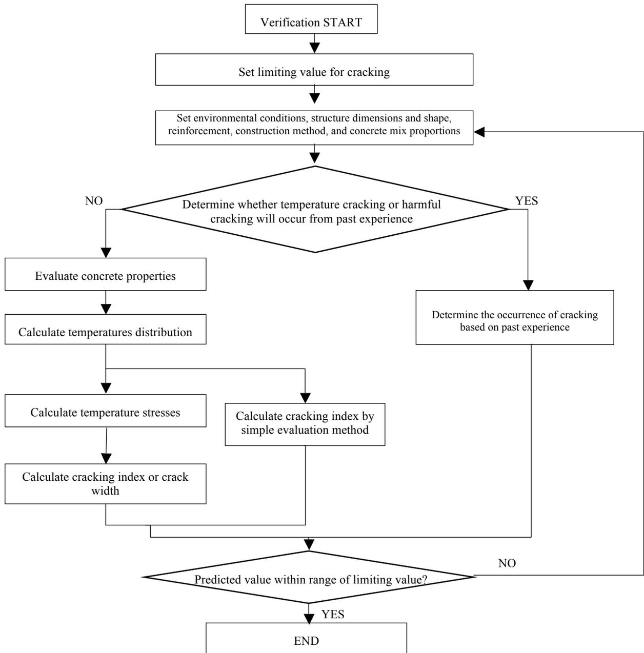
Fig. 1 Flow of temperature cracking verification
