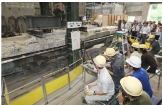
Fig.2 Loading test of real bridge girder
