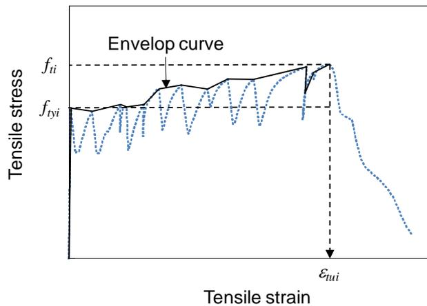
Figure 3 Method of tensile characteristics evaluation
