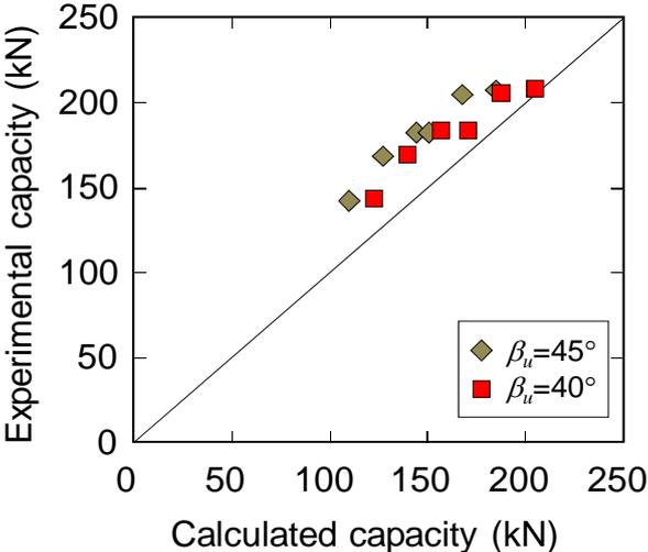
Figure 11 Comparison of experimental and calculated shear capacities
