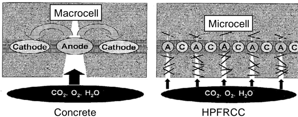
Figure 13 Differences of corrosion mechanism due to crack formation
