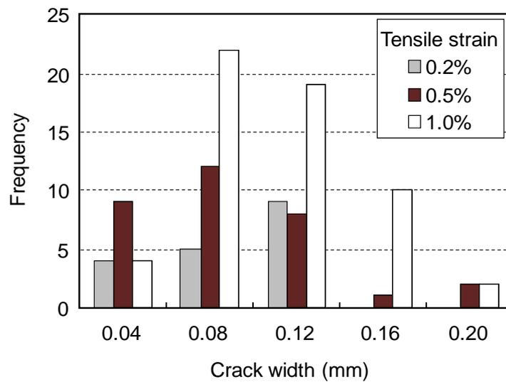
Figure 8 Distribution of measured crack widths at different tensile strain levels
