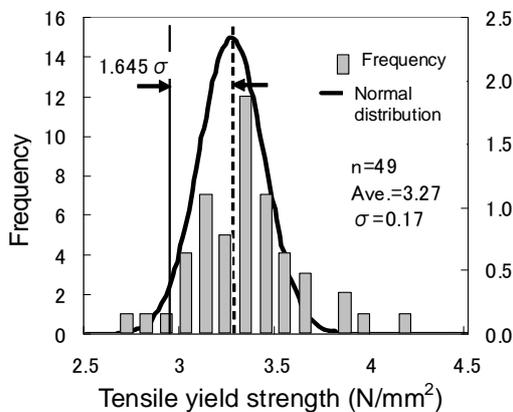
Figure 4 Variations in measured tensile yield strengths
