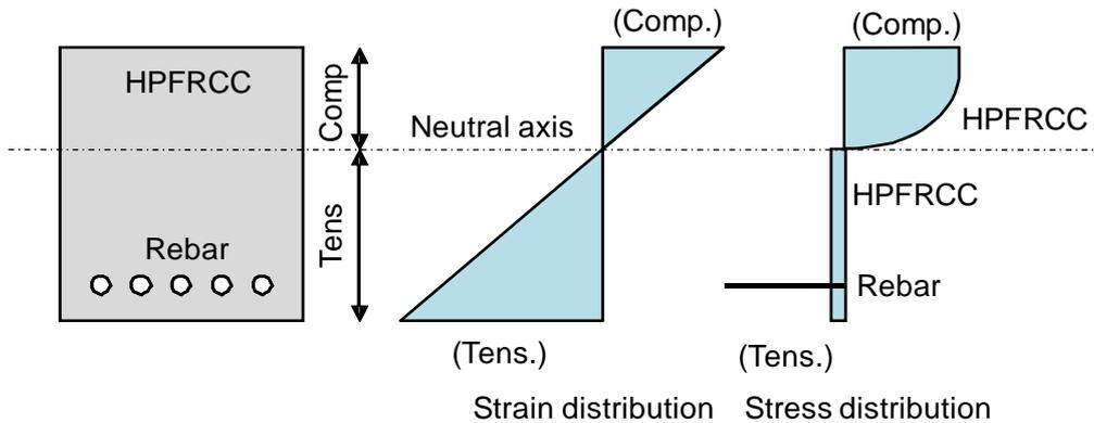
Figure 9 Schematic diagrams of strain and stress distributions for flexural capacity
