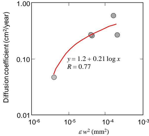
Figure 14 Example of measured chloride ion diffusivity
