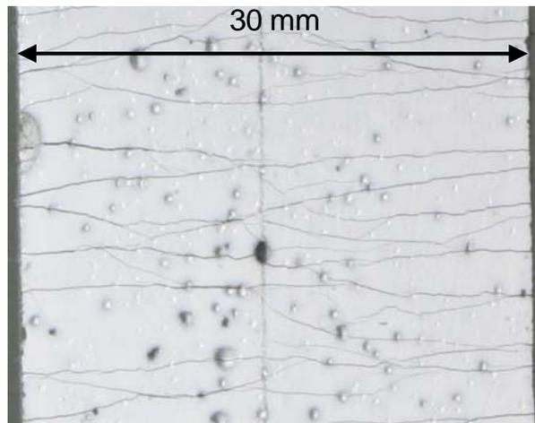
Figure 7 Multiple fine cracks in ECC
