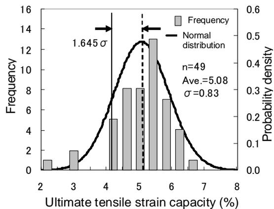
Figure 5 Variations in measured ultimate tensile strains
