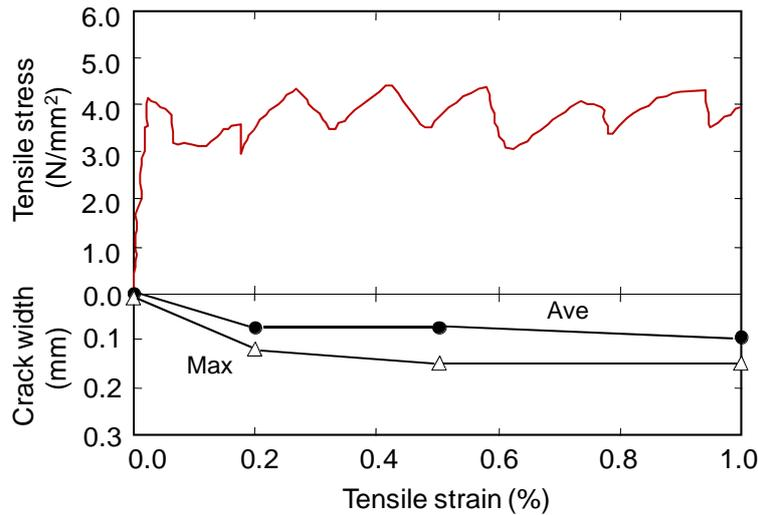
Figure 12 Effects of tensile strain on crack width
