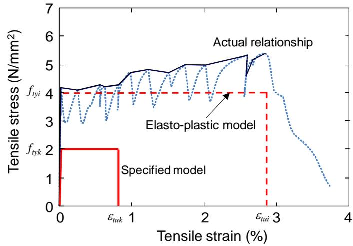
Figure 6 Models expressing tensile stress-strain relationships
