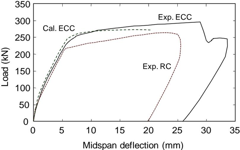
Figure 10 Examples of load-displacement curves
