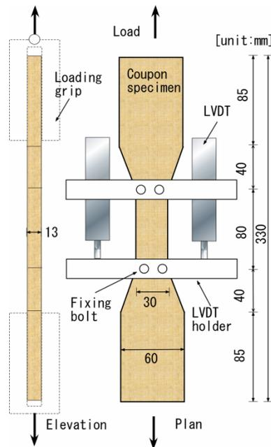
Figure 2 Test method for determining tensile characteristics
