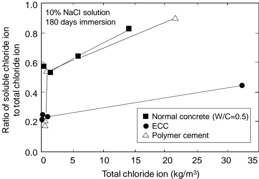
Figure 15 Example of permissible chloride ion concentrations for steel corrosion
