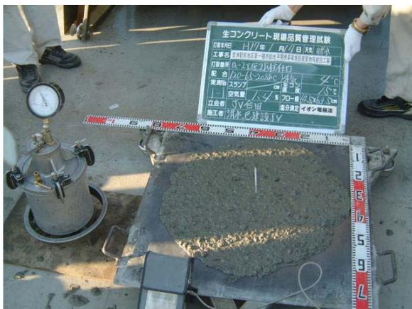
Fig. 34 Quality control tests
