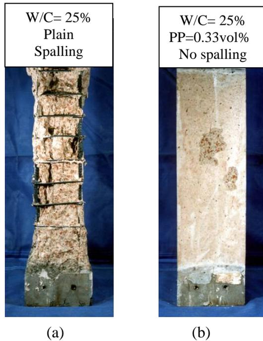
Fig. 10 RC columns after fire resistance test
