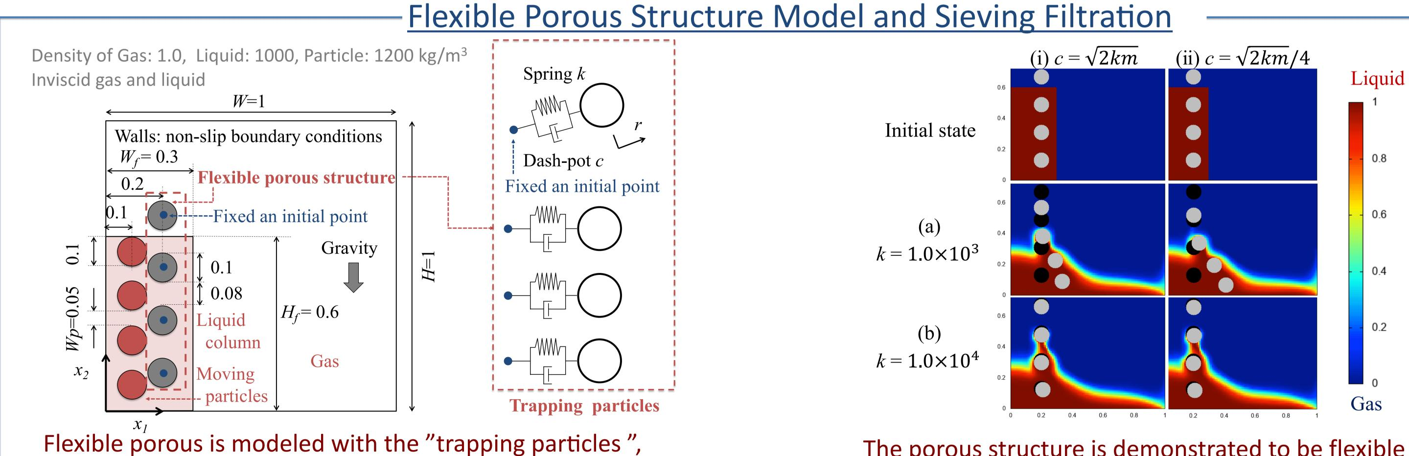
The porous structure is demonstrated to be flexible and connecting to its initial position with a spring and dash-pot. deformed depending on the spring k and dashpot c.
