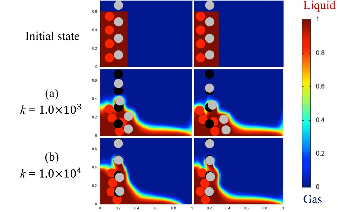
Sieving filtration is demonstrated numerically, retaining the "moving particles" by the "trapping particles".
