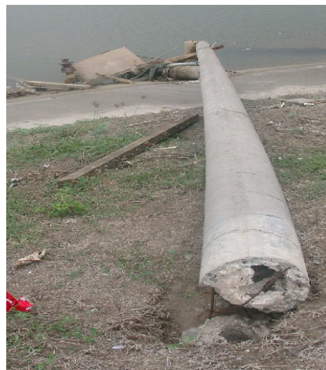
Photo 12.9 Broken electric distribution poles
