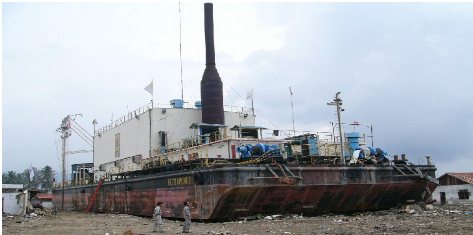
Photo 12.8 Displaced barge with a thermo-electric power generator
