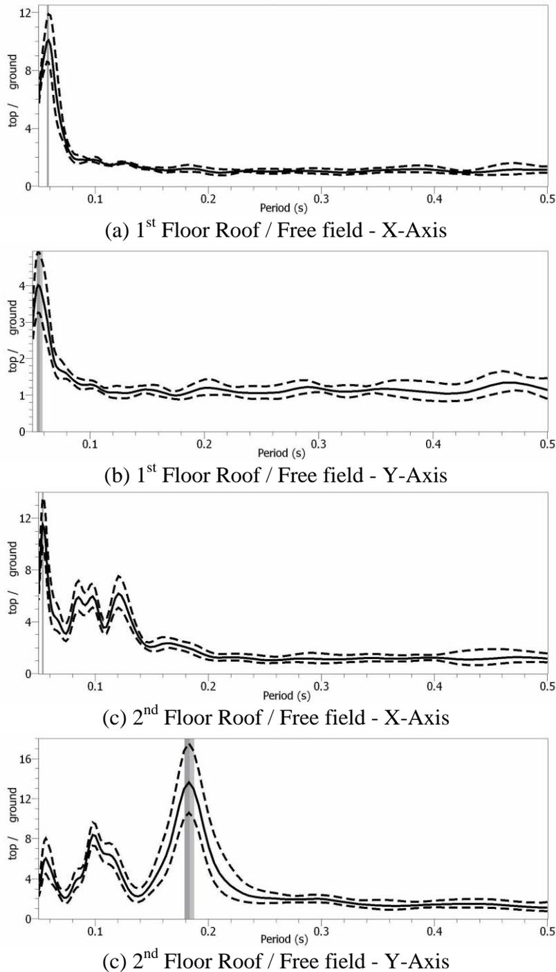
Fig. 4.76. Ratio of Fourier spectra of microtremor measurement in reinforced 2-story adobe house
