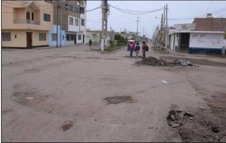
*Fig. 3.39. Central Pisco (S13 42.542 W76 12.516). Settled ground as evidence of broken sewer pipes.*
