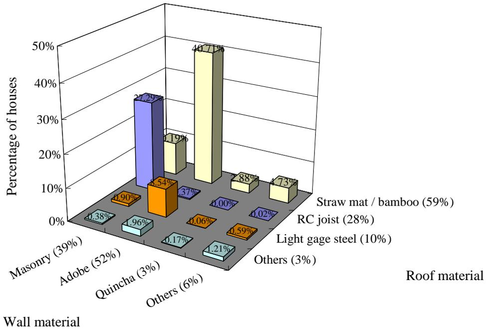
Fig. 4.13 Distribution of houses in the earthquake affected areas as of 2005 [1]
