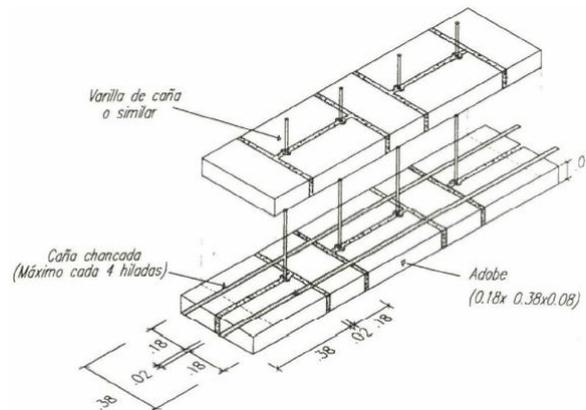
Fig. 4.70 Vertical and horizontal adobe reinforcement. After E.80 [11]
