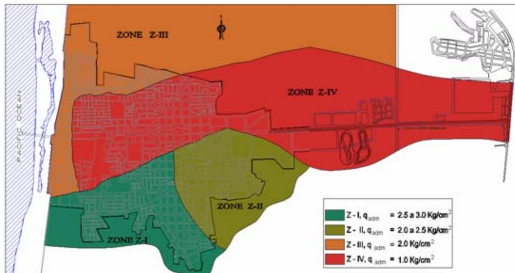
Fig. 3.35. Geotechnical zonation based on bearing capacity (Adapted from [13])
