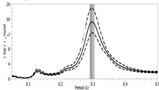
Fig. 4.56 Microtremor measurement analysis results (Transverse direction)
