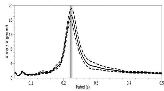
Fig. 4.57 Microtremor measurement analysis results (Longitudinal direction)
