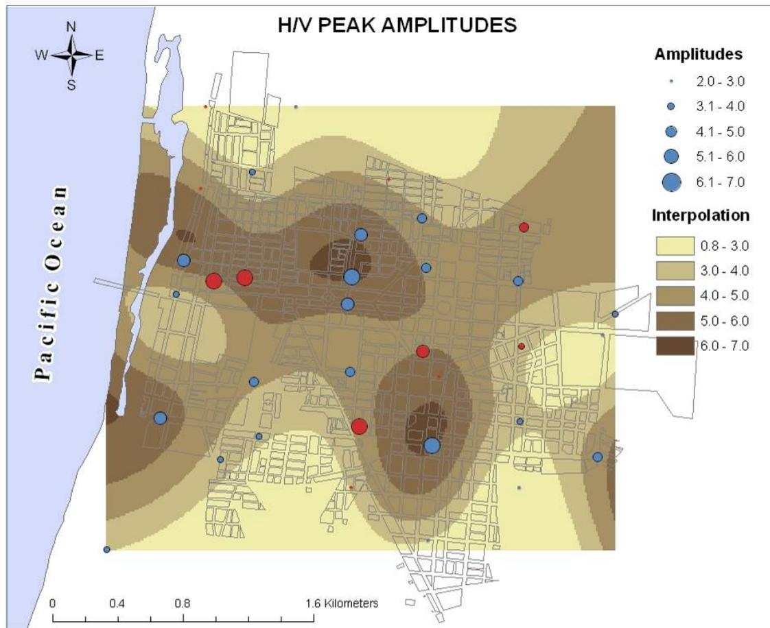
Fig. 3.59. H/V peak amplitudes. Local values and contours.
