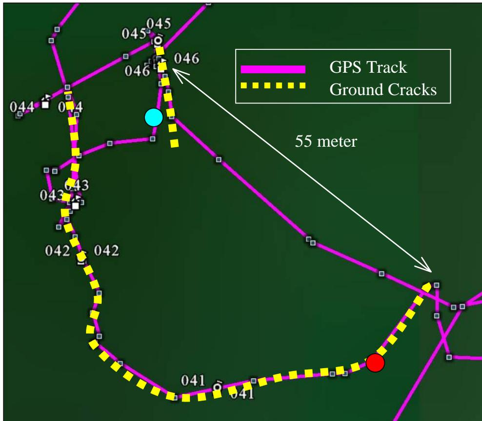
Fig. 3.6. Close up of ground cracks and GPS tracks at point 41-46. Photos taken at light blue dot and red dot are shown in Fig. 3.7 and Fig. 3.8. Cracks were some 70 meters long.
