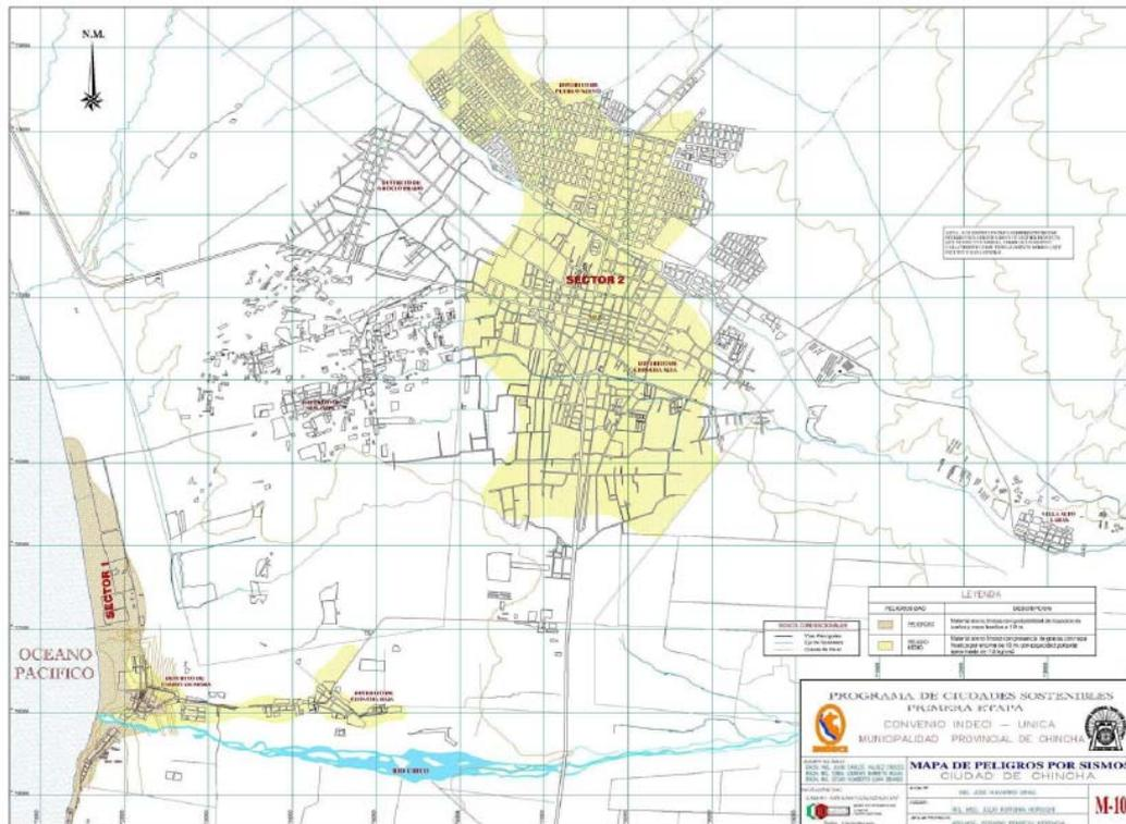
Fig. 3.24. Seismic Hazard Areas City of Chinchipe. INDECI [1]. Brown colored area next to the ocean indicates “dangerous” area.
