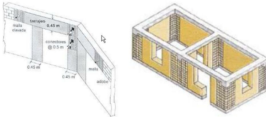
Fig. 4.64. Wire mesh reinforcement. After Blondet [9]
