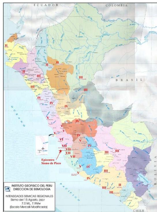
Fig. 2.4. Modified Mercalli intensities according to the Institute of Geophysics of Peru. [1].
