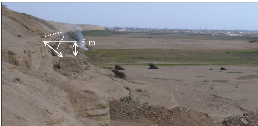
*Fig. 3.34. Block moved seemingly moved down and towards ocean some 5 meters, however there was vegetation between the block and the slope, so this did not happen in the 2007 earthquake.*
