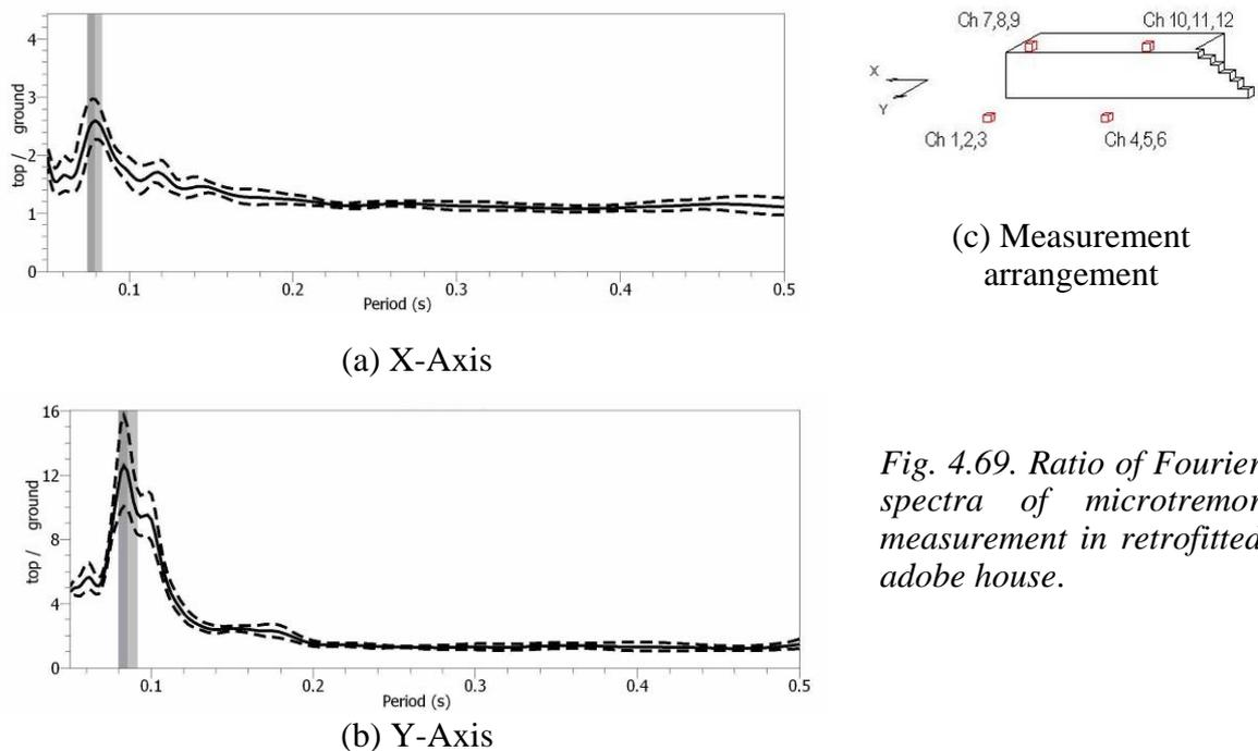
Fig. 4.69. Ratio of Fourier spectra of microtremor measurement in retrofitted adobe house.
