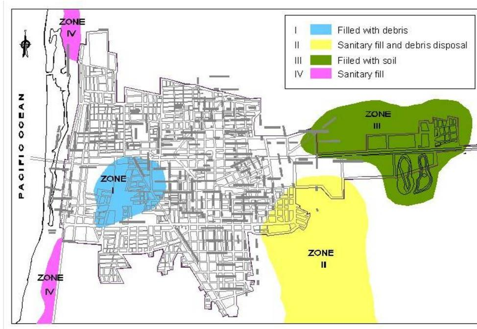
Fig. 3.38. Distribution of landfills in Pisco (Adapted from [13])
