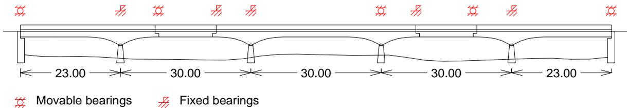
Fig. 5.16 Layout of the Huamani bridge (downstream direction)
