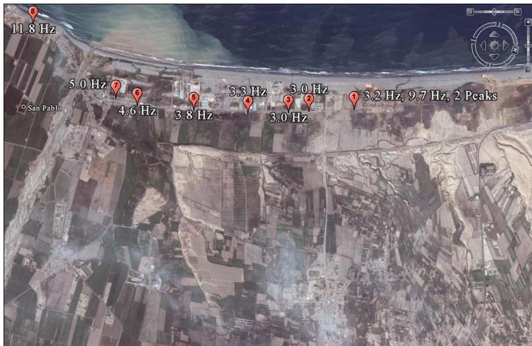
Fig. 3.32. Google earth image of microtremor measurement locations and results.
