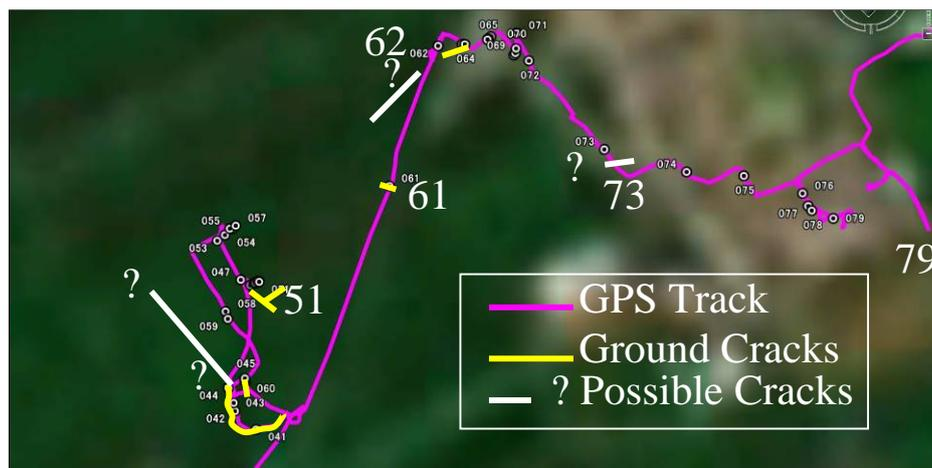
Fig. 3.5. Google earth view of San Luis Annex Nuevo Monterrico with GPS tracks in purple. Yellow shows location of large cracks. White shows location of cracks reported by local people. White colored crack located close to point 62 we observed from the road only.
