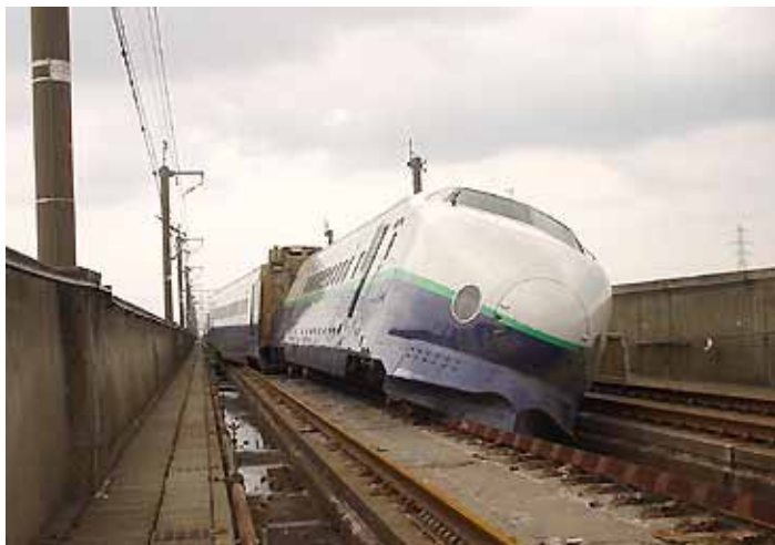
Fig. 2. Derailed train of Shinkan-sen in the Oct. 23, 2004, Chuetsu Earthquake.
