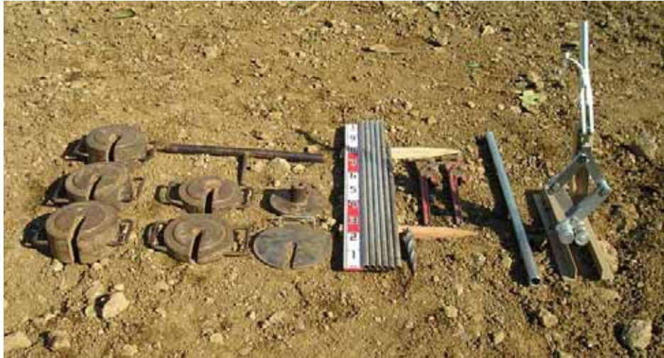
Figure 4. Equipment of the Swedish Weight Sounding Test
