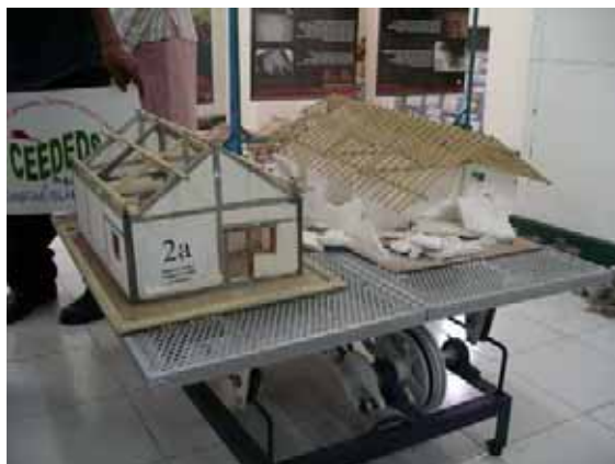
Photo12 Demonstration of the different failure mode between brick wall house confined by RC frame(left) and usual unconfined brick wall house(right) on the shaking table at Indonesian Islam University
