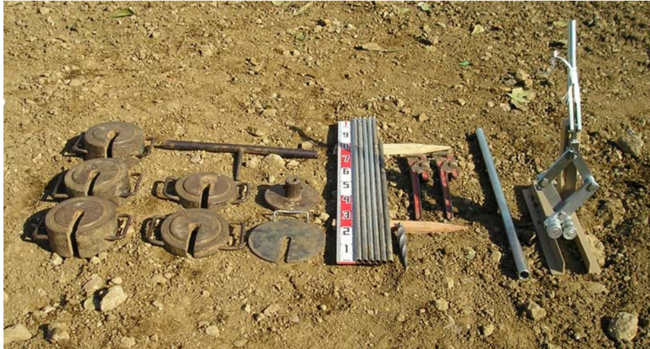
Figure 4. Equipment of the Swedish Weight Sounding Test
