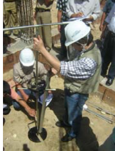
Training on ground survey methods with Swedish Weight Sounding Test (Gunung Sitoli)
