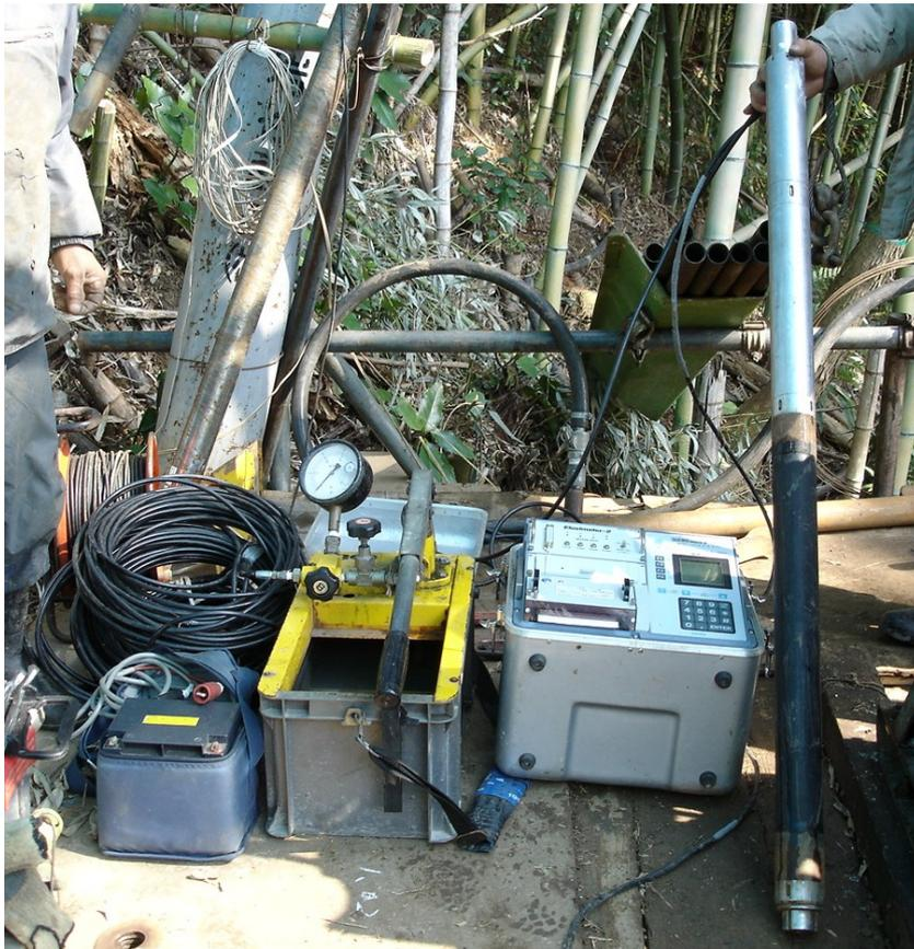
Figure 11.30 A view of elastometer (pressuremeter) test
