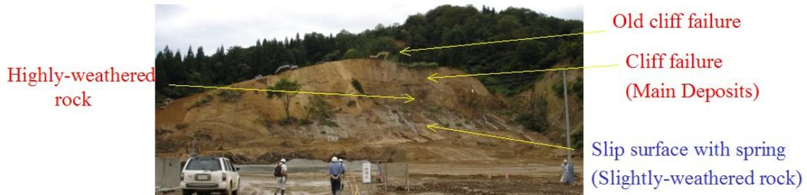
Figure 11.27 An example of outcrop survey of a landslide area
