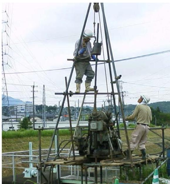
(a) Standard penetration index test set-up
