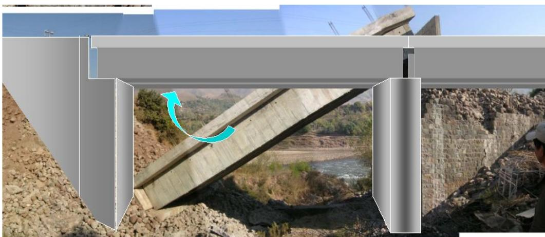
Figure 11.3 New bridge recommendation for the damaged bridge with the use of existing girder
