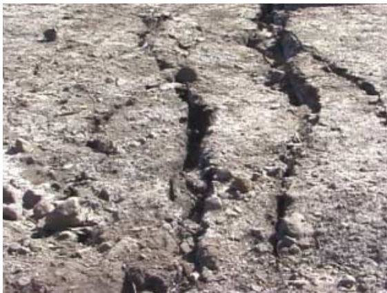
(c) Cracking in ground surface located at a horizontal distance of about 25 m from drainage channel
