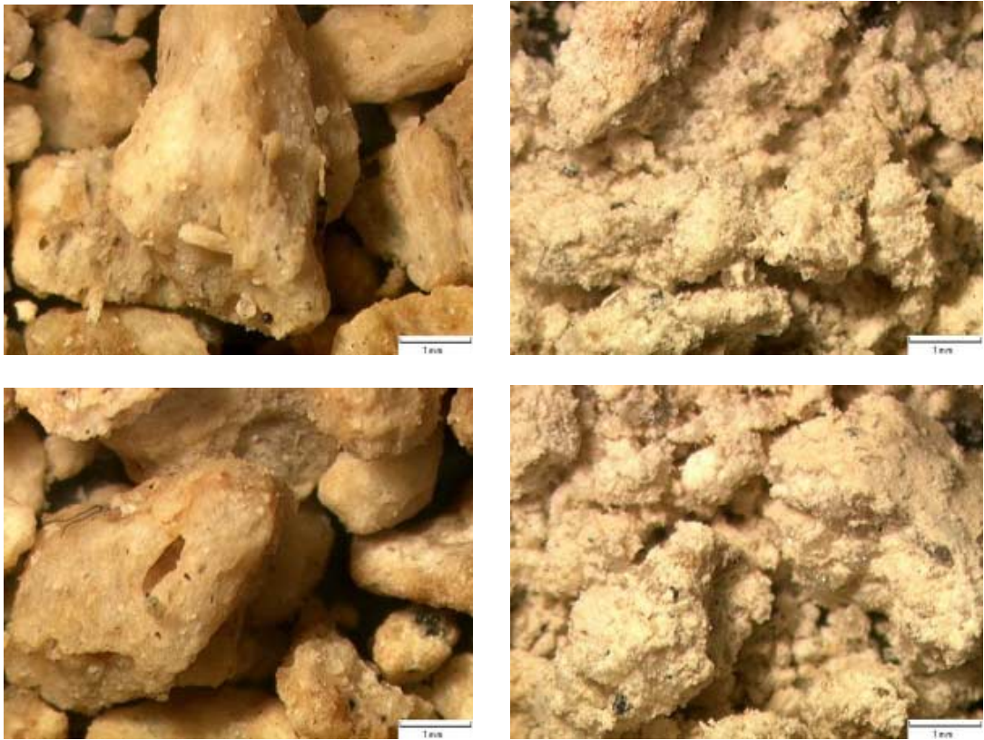
Figure 2.45. microstructure of the pumice by optical microscope (Left: before the test, Right: after the test)
