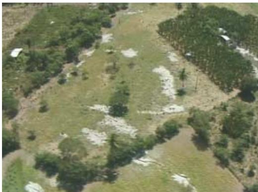
**Figure 5.16** Liquefaction-induced sand boils along Lempa River
