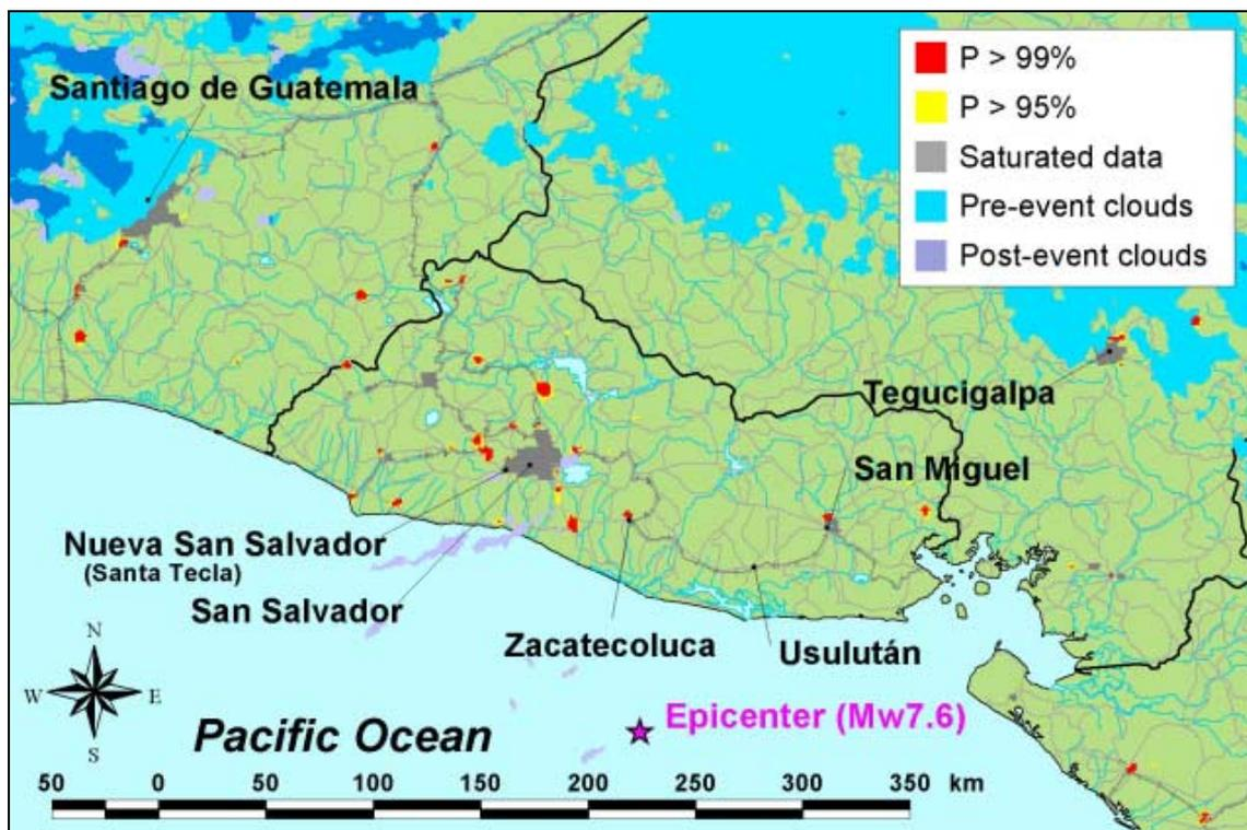
Figure 5.9 Estimated damaged area using two images on January 12 and 14.
