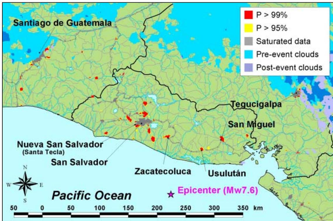
Figure 5.8 Estimated damaged area using two images on January 12 and 13.
