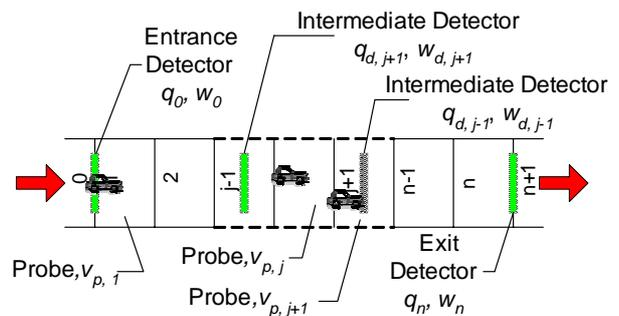
**Figure 2** Road section with probe vehicles and fixed detectors
