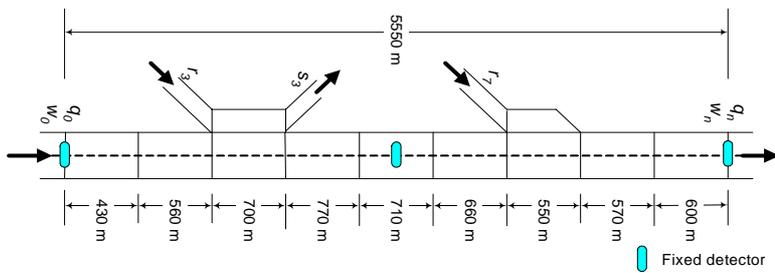
Figure 3 Geometry of the studied road section
