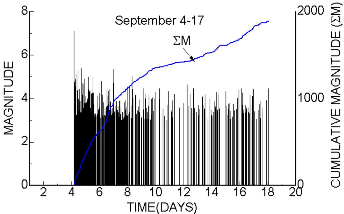
Figure 11: Time series of magnitude and cumulative magnitude in the epicentral area during the post-seismic activity between September 4 and 17, 2010
