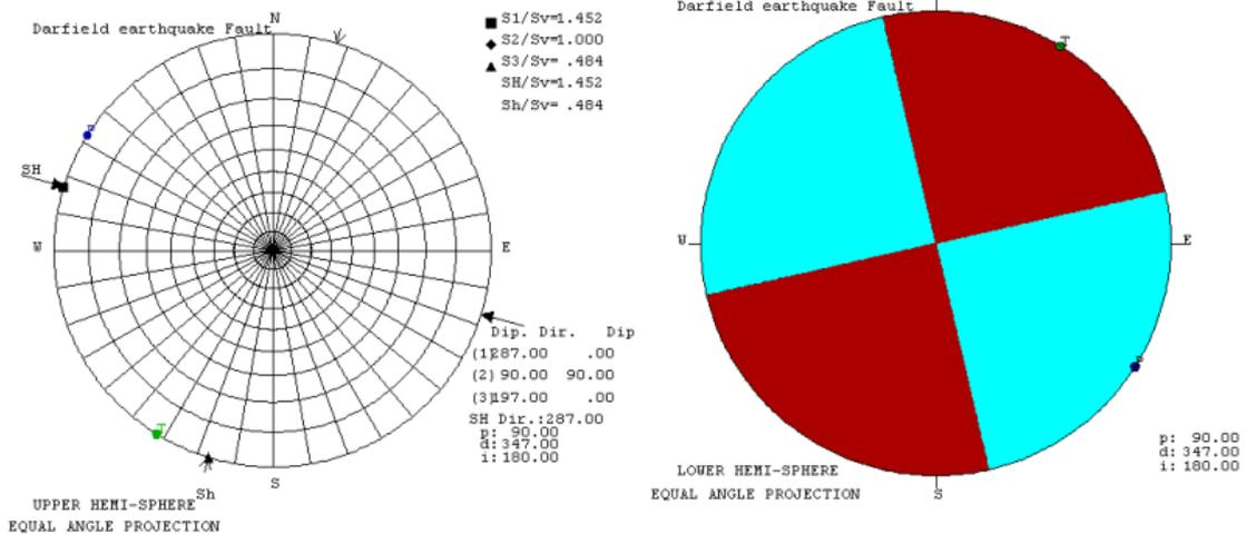
Figure 13: The stress state and focal mechanism of the earthquake inferred from Aydan's method
