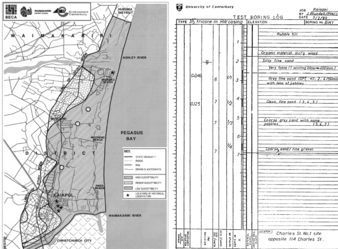
Figure 22: Ground liquefaction potential at Kaiapoi (arranged from Berrill et al., 1994)
