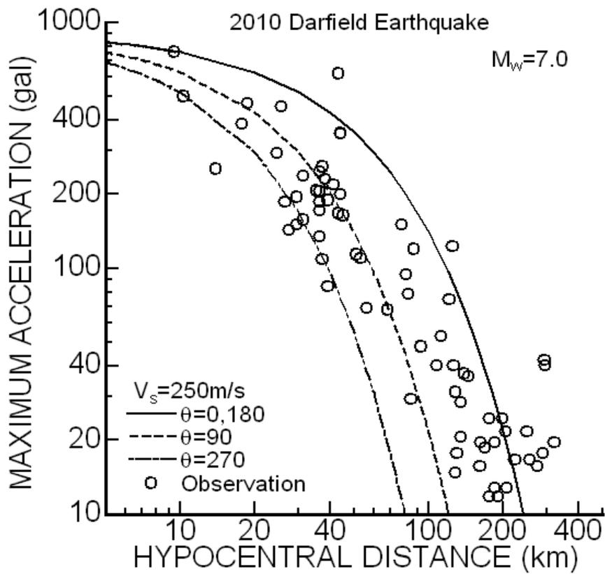
Figure 16: Attenuation of maximum ground acceleration
