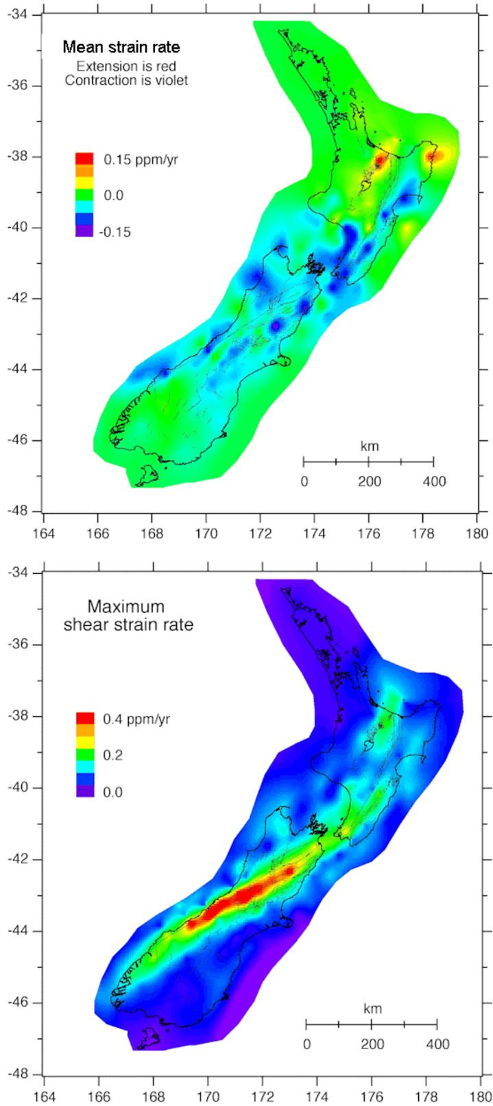
Figure 6: Mean and maximum shear strain rates for 2003 (from GNS)
