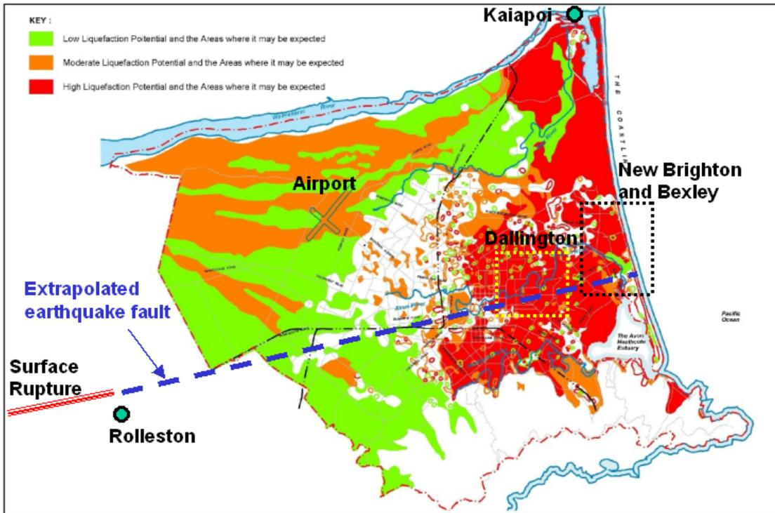
Figure 21: Liquefaction potential in Christchurch (modified from City Council)
