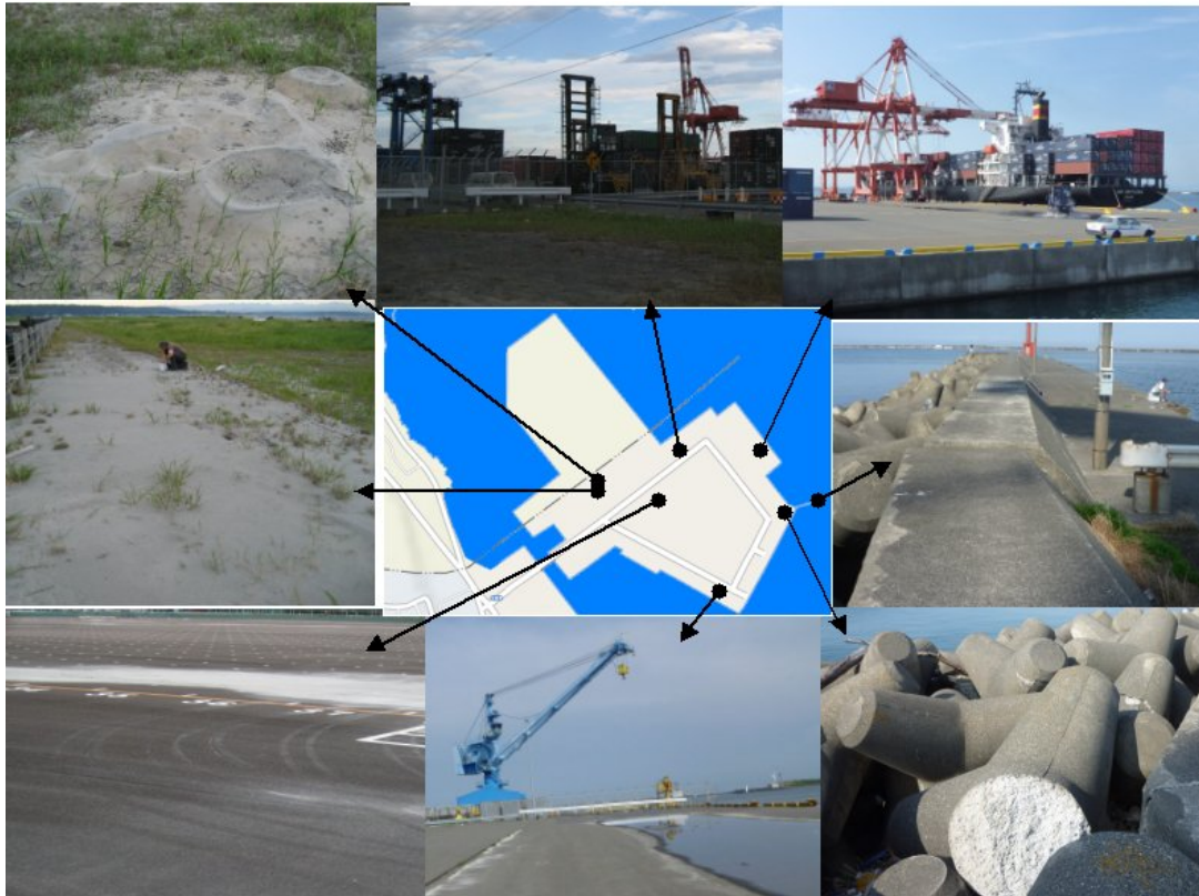
Figure 51: Damage at the west wharf of Omaezaki port on reclaimed land
