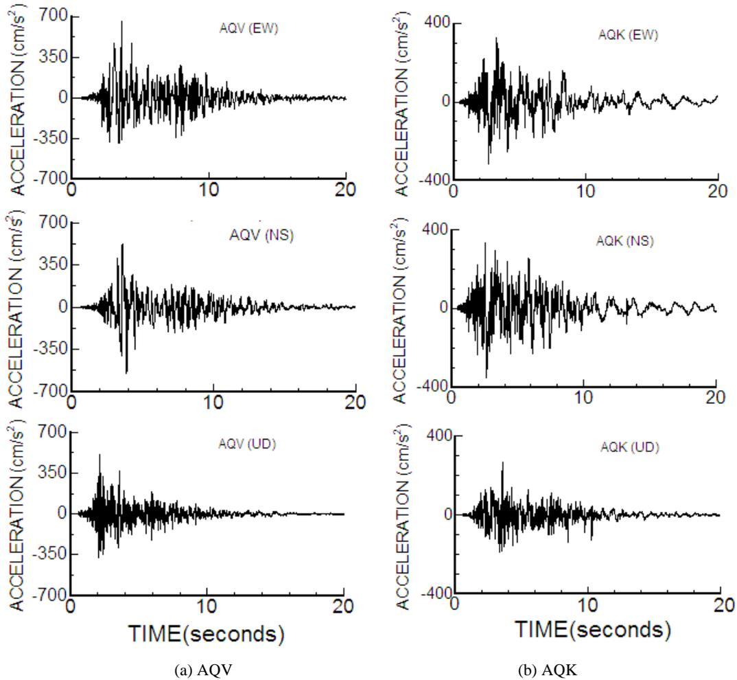
Fig. 2 Acceleration records at AQV and AQK stations
