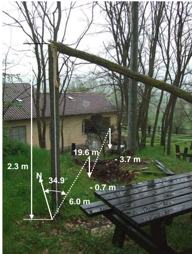
**Photo 5** A broken tree, a shallow dent on the ground and a collapsed wall of the building along the path of a fallen rock.
