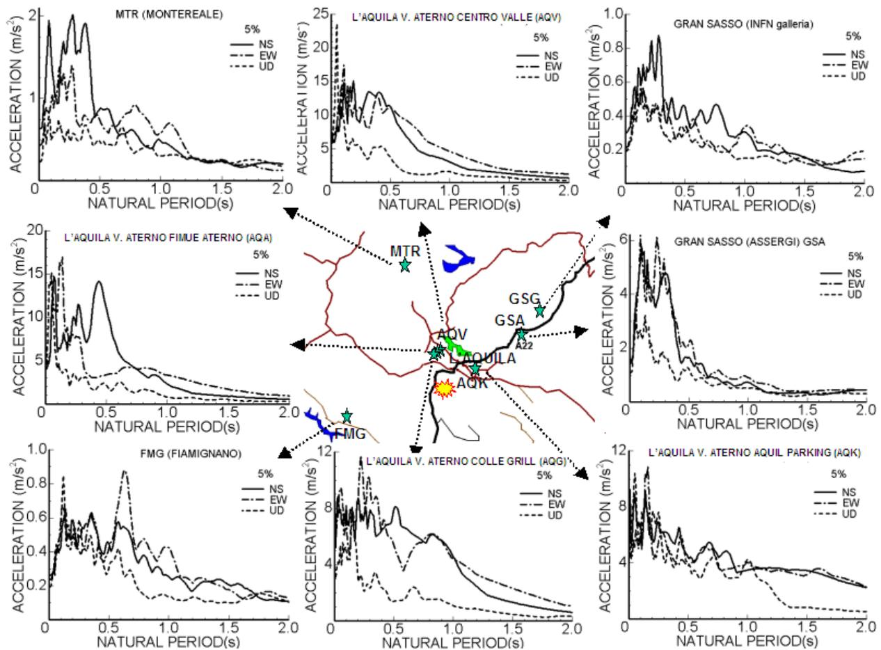
**Fig. 3** Acceleration response spectra of selected strong motion stations
