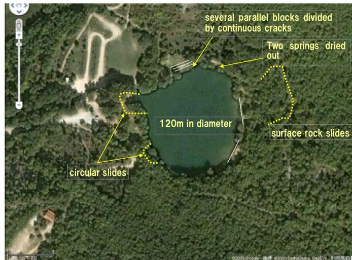
**Photo 1** Lateral spreading around Lake Sinizzo (added on Google map)
