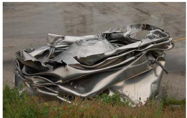
Photo 36 Buckled bottom of a silo
