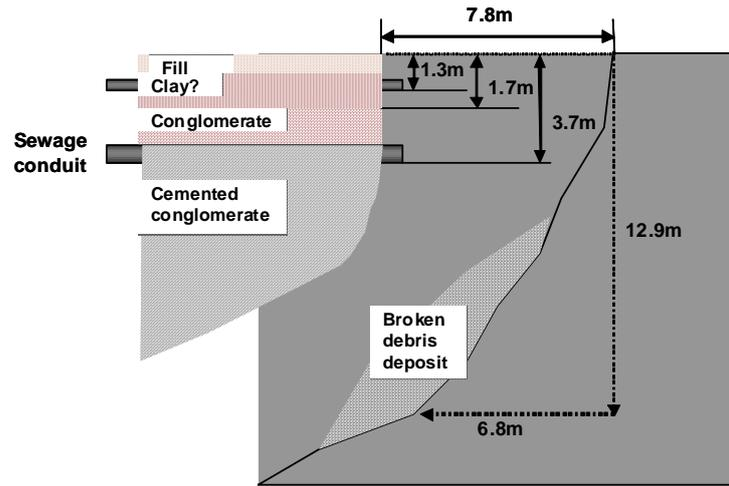
Fig. 4 Section of a sinkhole (Refer to Photo 7)
