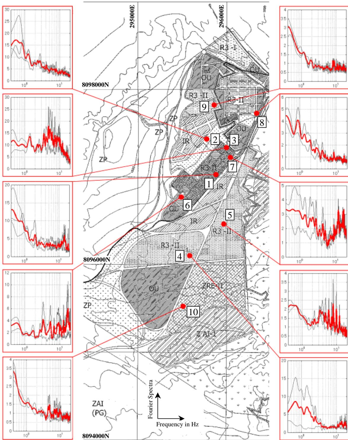
**Figure 3.8** Microtremor measurements at Chechen – EW Component Fourier Spectra
