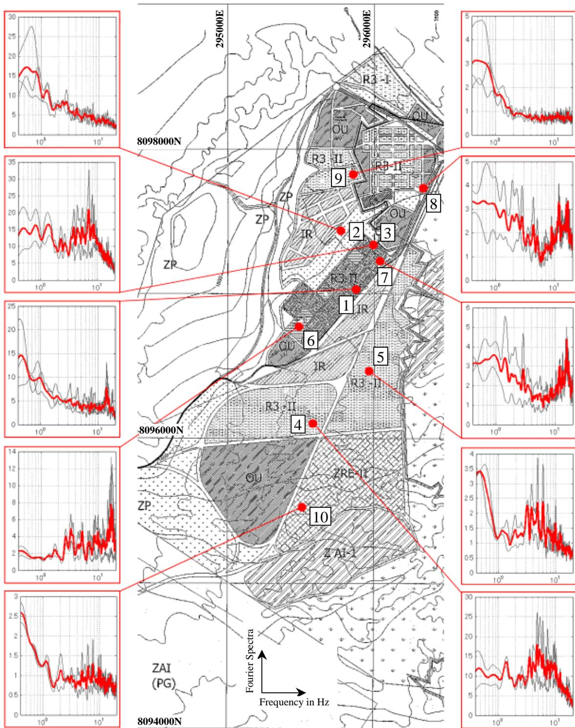
**Figure 3.7** Microtremor measurements at Chechen – NS Component Fourier Spectra
