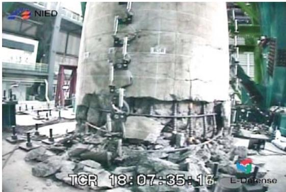
▲ A bridge column designed in accordance with the design requirements in the 1970s.
