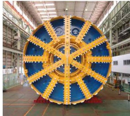
Tunnel Boring Machine (TBM)
