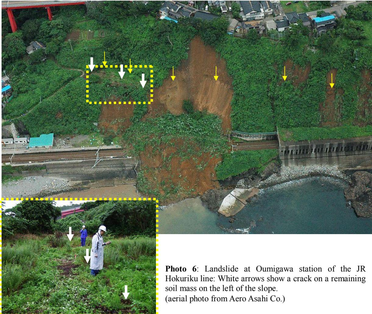
**Photo 6:** Landslide at Oumigawa station of the JR Hokuriku line: White arrows show a crack on a remaining soil mass on the left of the slope. (aerial photo from Aero Asahi Co.)
