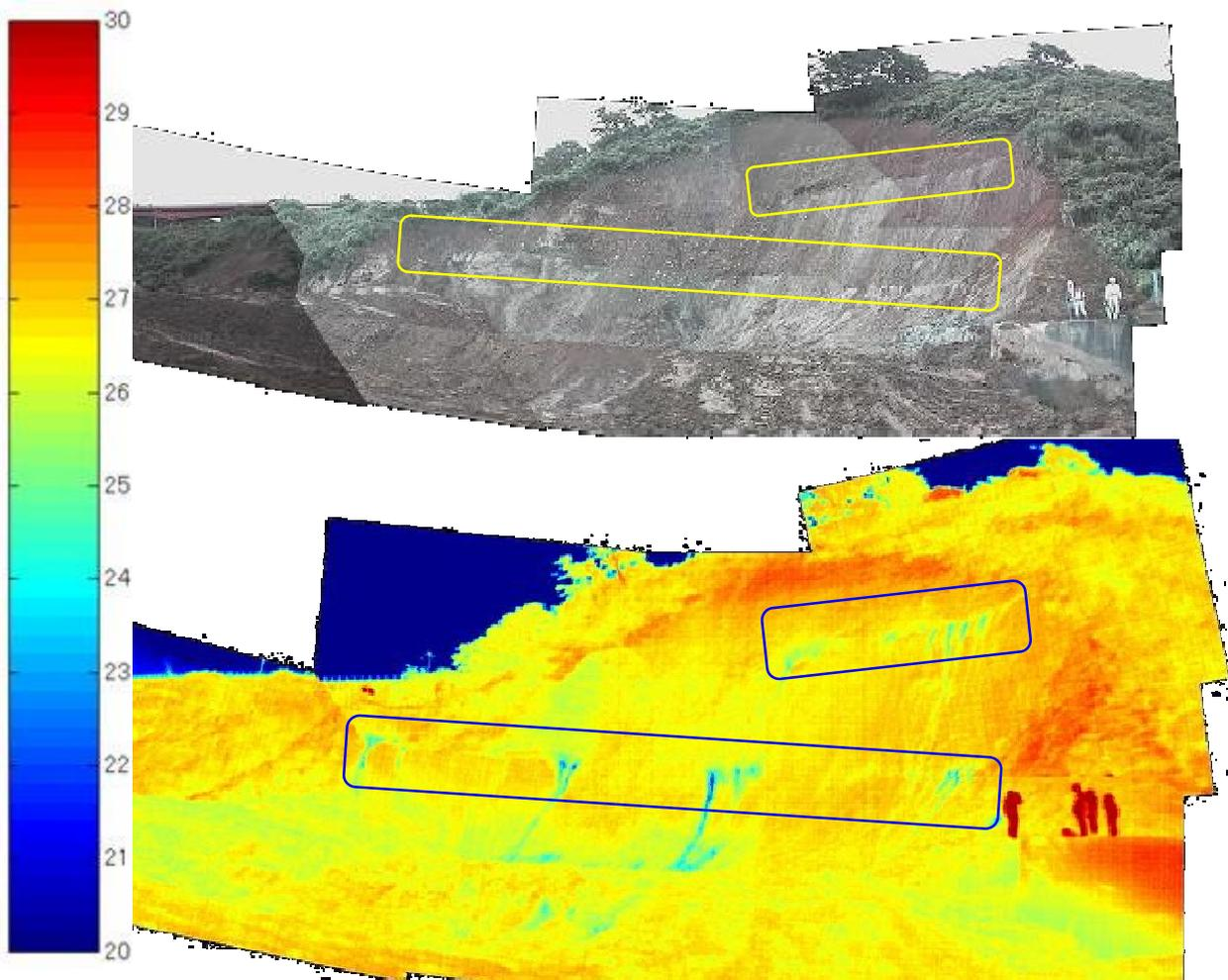
**Photo 9:** (a) normal and (b) Infrared image of slope surface. Color scale shows “degrees” on Celsius temperature scale.
