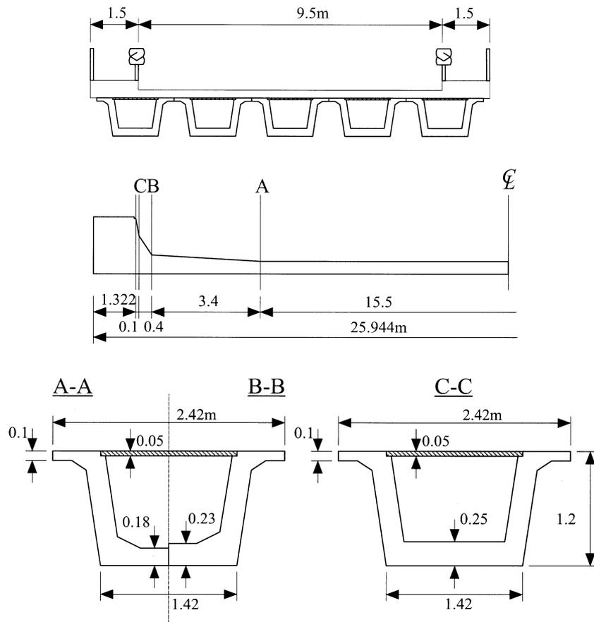
Fig. 5.4 Deck Section, Arifiye Overpass
