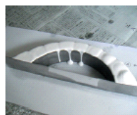
Photo 2 Pouring gypsum into the forms
