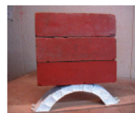
Photo 4 Heavy bricks placed on the arch
