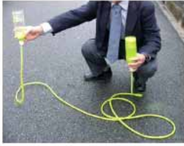
Photo 32 A level made of PET bottles and a vinyl hose
