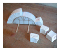
Photo 3 Assembling arch blocks
