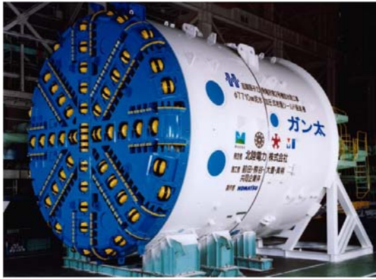
Photo 5 : The slurry type shield machine designed for rock
