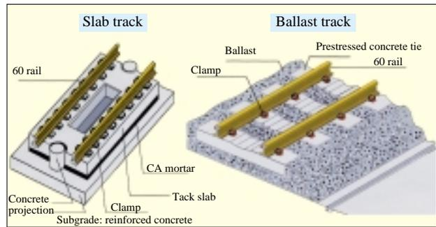
Fig. 8 Slab track and ballasted track
