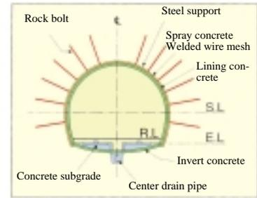
Fig. 5 Standard NATM support arrangement
