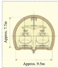
Fig. 4 Typical tunnel section
