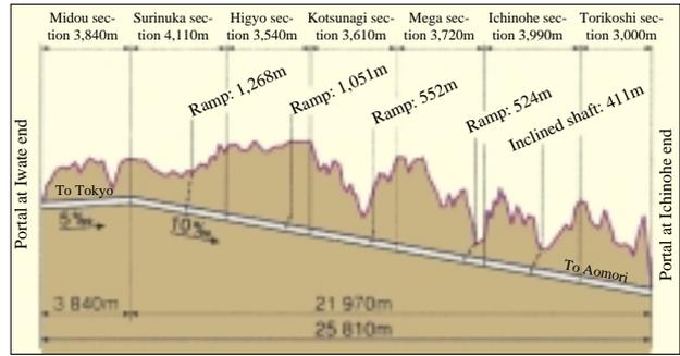
Fig. 3 Longitudinal section of tunnel showing construction sections
